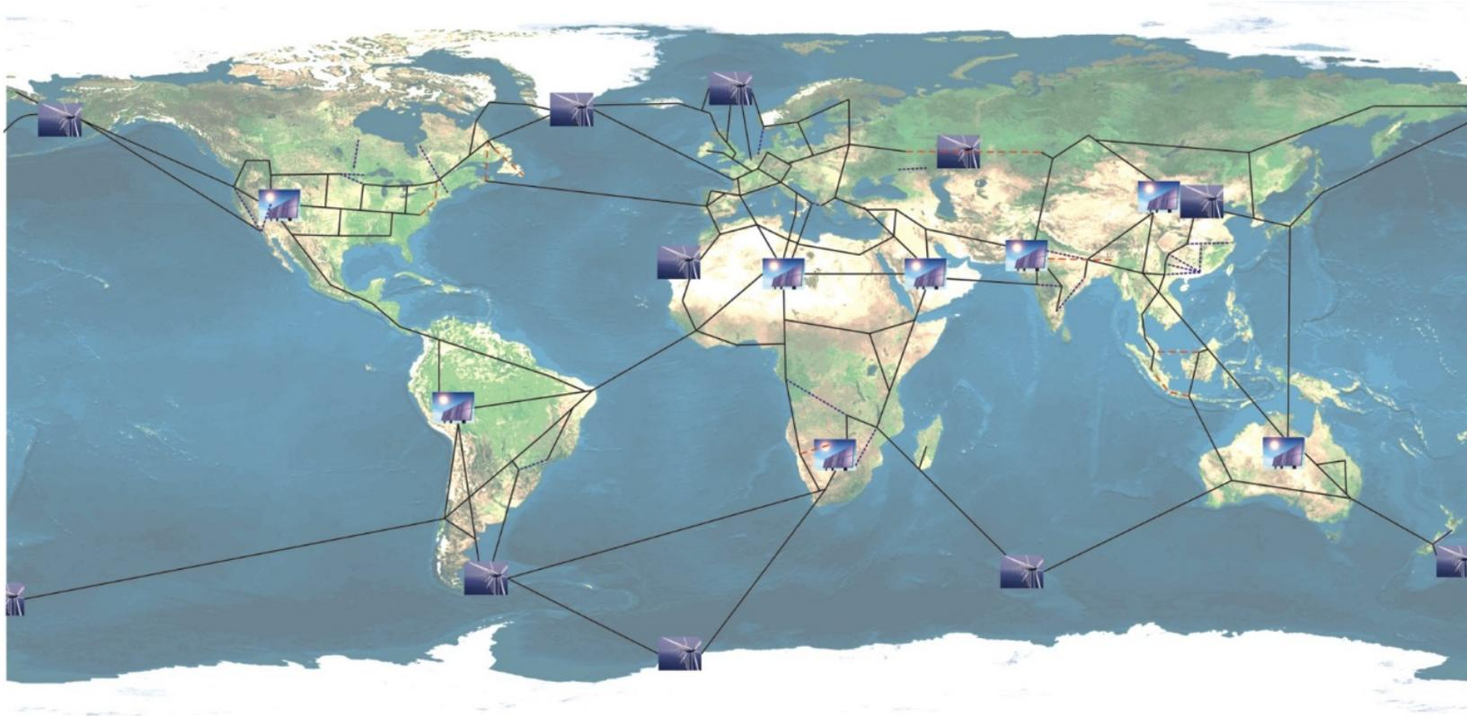
A **global (green) grid** is an electrical network spanning the whole planet and connecting together the world's consumers and producers of electricity. Its backbone would be made of (very long) High Voltage Direct Current (HVDC) links.
