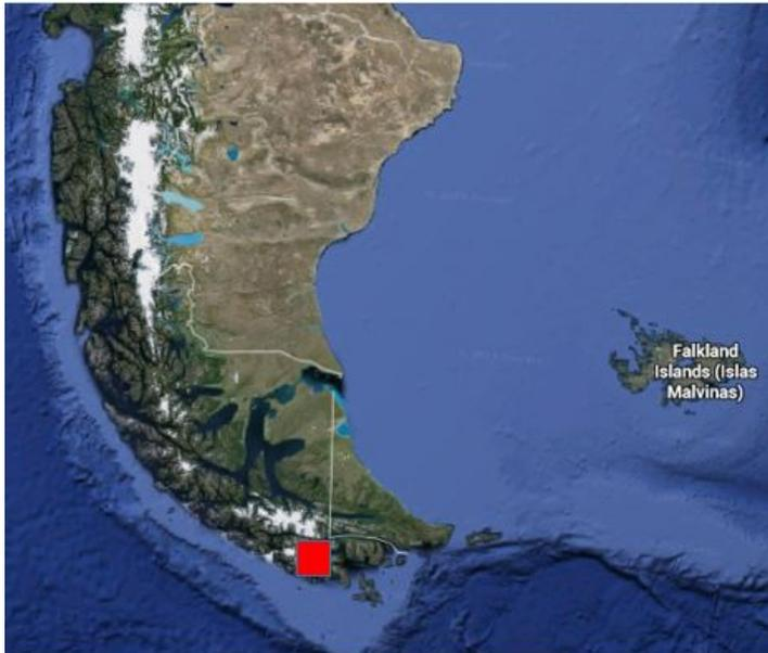
A wind farm in the southern part of South America can generate  $13 \text{ W/m}^2$ , against  $3 \text{ W/m}^2$  in mainland Europe. The total consumption of electricity in Brazil, which is around 500 TWh/year, could be generated by covering the red area on this map with wind mills.
